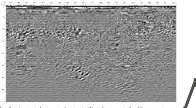
Data illustrates a terminal end moraine deposit with visible stratigraphy greater than 375 nanoseconds.
